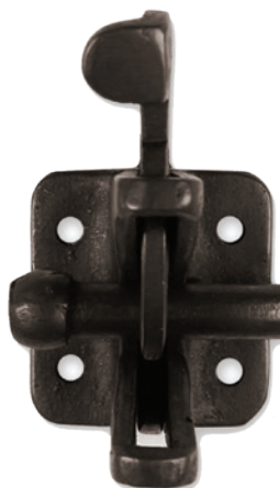
Standard Gate Latch - Straight 50-200 Dimensions: 2" L x 2" W x 1-3/4" H Catch: Straight Screw: 1" Round | #10 Stainless
